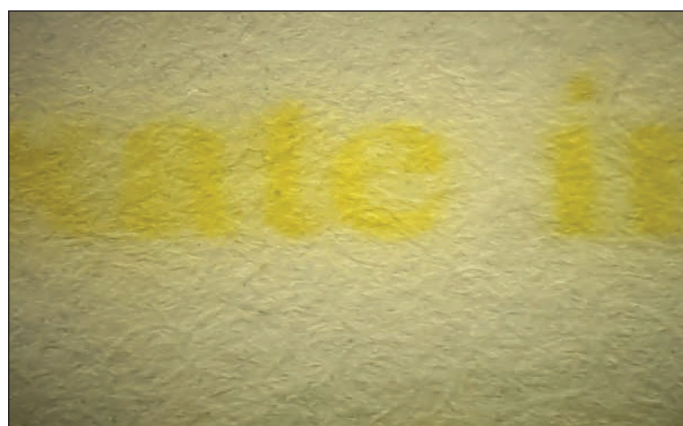
Figure 4. Change in the texture of bond paper and spreading ink after immersion in neutral medium for fifteen days.
