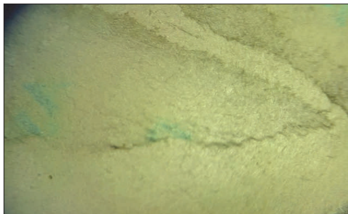
Figure 3. Change in the texture of A4 plain paper after immersion in acidic medium for one month.
