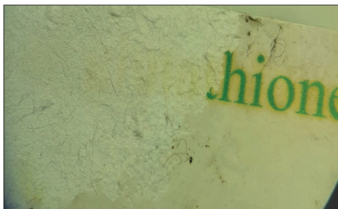
Figure 2. Change in the texture of glossy paper after immersion in acidic medium for fifteen days.
