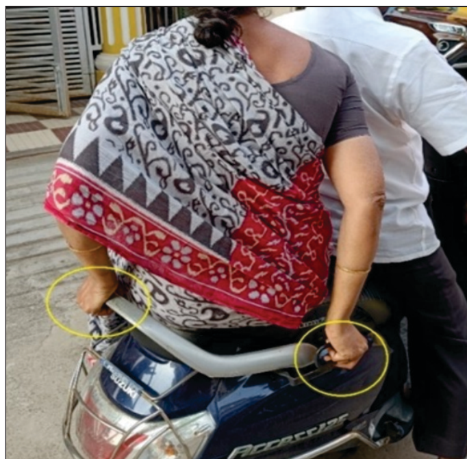
Figure 4: Inconvenient provision of handles for pillion rider (yellow circle).
