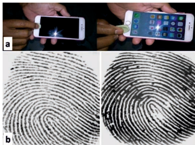
Figure 3: a: Unlocking of mobile using alginate finger. b: Scanned image derived from optical sensor device showing higher intensity of the fingerprint by alginate finger than the sample finger of the same person.
