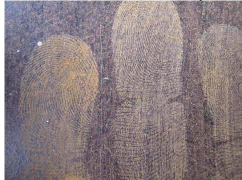
Fig 9: Showing the development of fingerprints on white A4 size paper after 5 days
