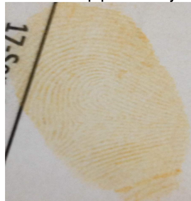
Fig 9: Showing the development of fingerprints on white A4 size paper after 5 days
